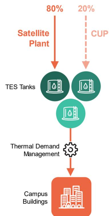
Figure 2-10: Chilled Water Supply Diagram
