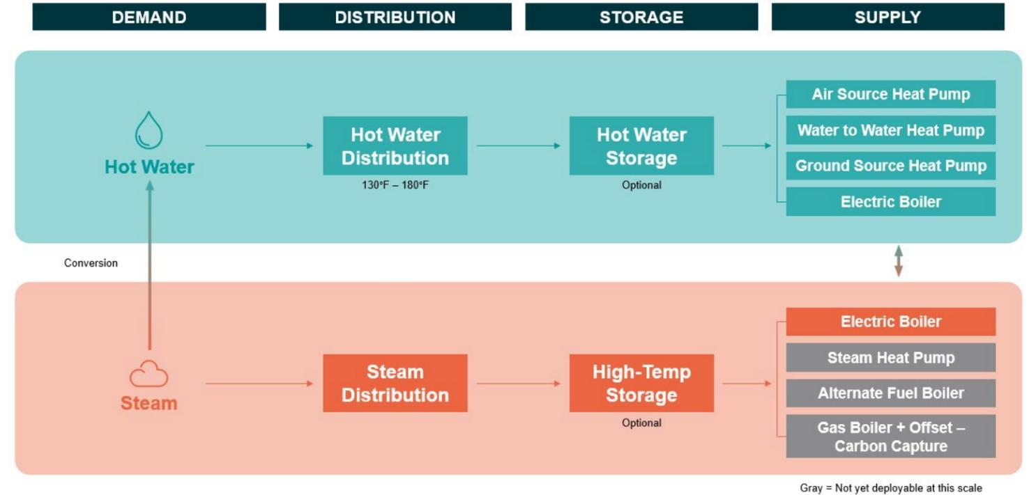
**Figure 3-1: Summary of Centralized System Decarbonization Technologies**
