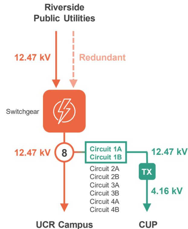
Figure 2-3: Electricity Supply Diagram
