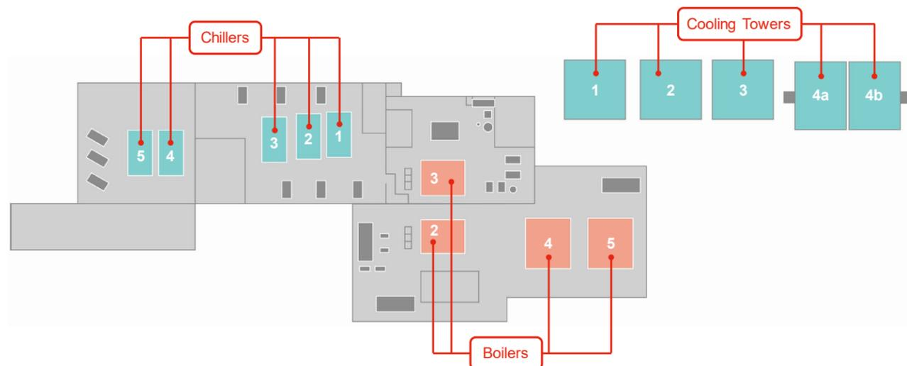
**Figure 2-13: CUP Equipment Layout**
