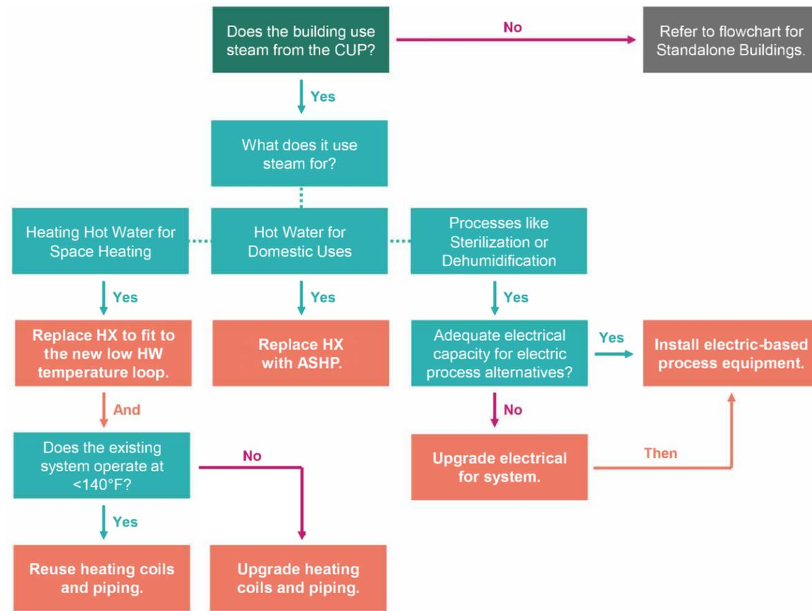
Figure 4-3: Building Upgrade Decision Flowchart for Connected Buildings
