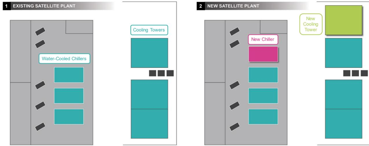
Figure 4-5: Satellite Plant Upgrades of the Featured Scenario
