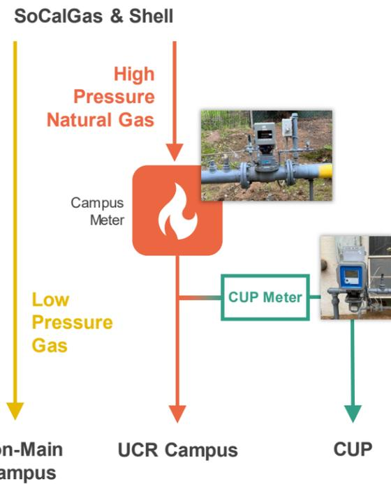
Figure 2-5: Natural Gas Supply Diagram
